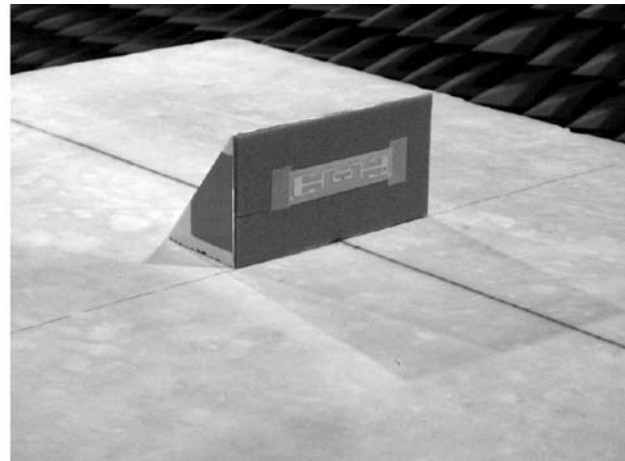
Fig. 5. Two different tags placed on a water container with a spacer of 2 mm and a metal surface with a spacer of 4 mm
